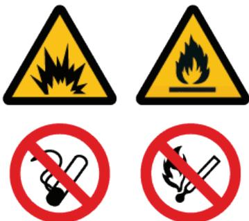
Do not smoke or allow smoking near fuel or the tool, or while using the tool. Mix and pour fuel outdoors and where there are no sparks or flames.
