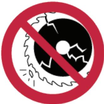
**Do not use dull or damaged cutting blades.**
