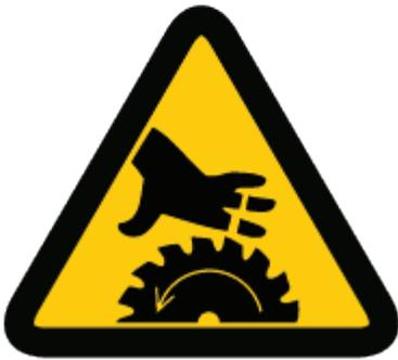
**Keep all parts of your body away from cutting attachment when the engine is running.**
