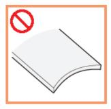
Do not rip workpiece that is twisted, warped or does not have a straightedge to guide it along the fence.
