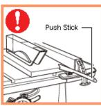
Always use a push stick for small pieces of wood and for pushing stock past the blade.
